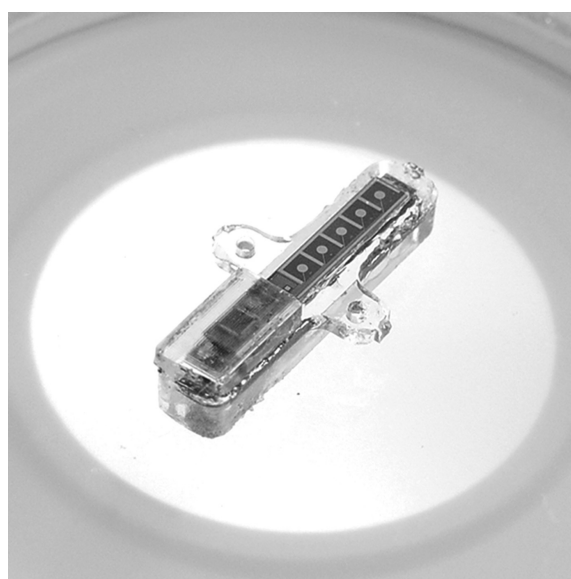
Figure 42.1 The i-IronIC implantable sensor. Courtesy of S. Carrara.
